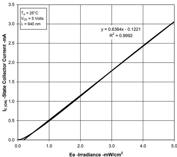
Collector Current Vs Collector to Emitter Voltage vs Irradiance
