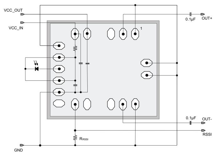
Figure 15. Basic Application Circuit for PIN Receivers
