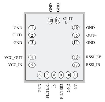
Figure 2. Bond Pad Assignment of ONET8521T
