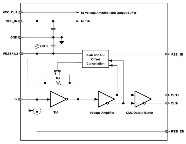
Figure 1. Simplified Block Diagram of the ONET8521T
