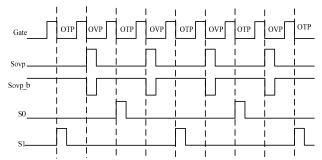
On-Bright proprietary dual function of external OTP and output OVP provides feasible and accurate detection of external OTP through NTC resistor and output OVP. The dual function is realized through time-division technology as shown in the figure.
