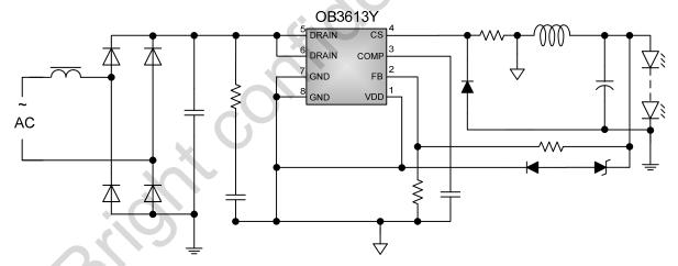
Figure 1: OB3613Y Typical Application Schematic
