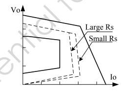
Fig. 2 Adjustable output power by changing Rs
