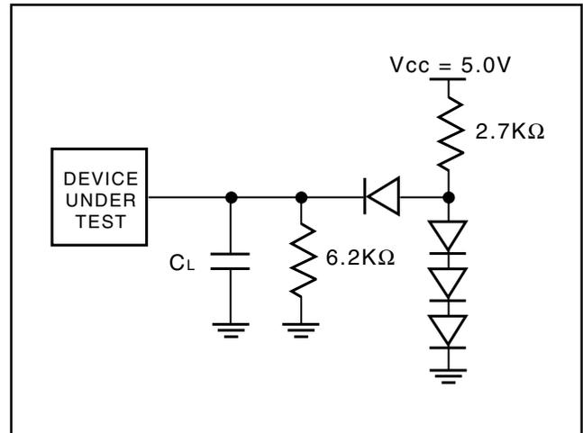
Figure 12. Test Setup
