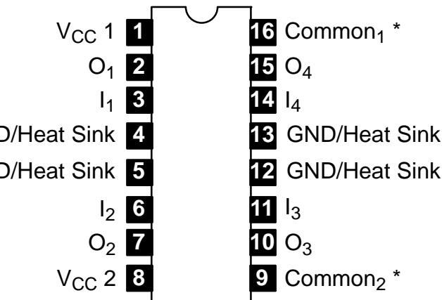
**Note:** These pins are internally connected.
