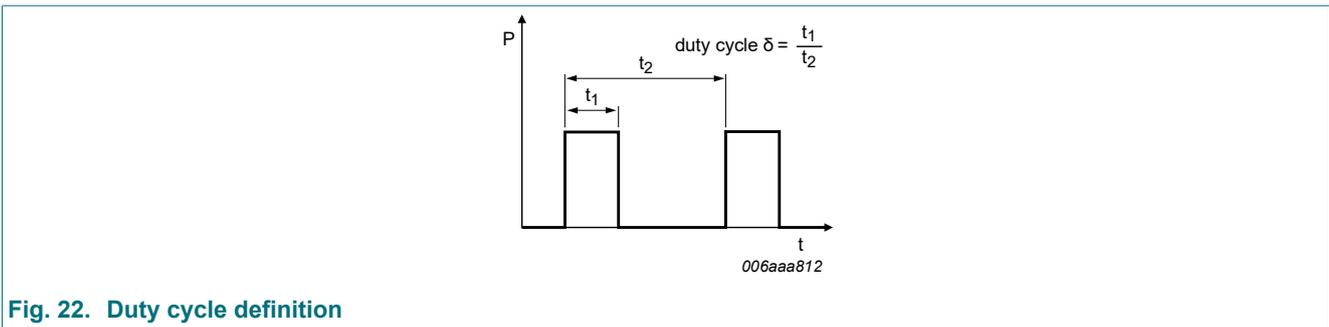
Fig. 22. Duty cycle definition
