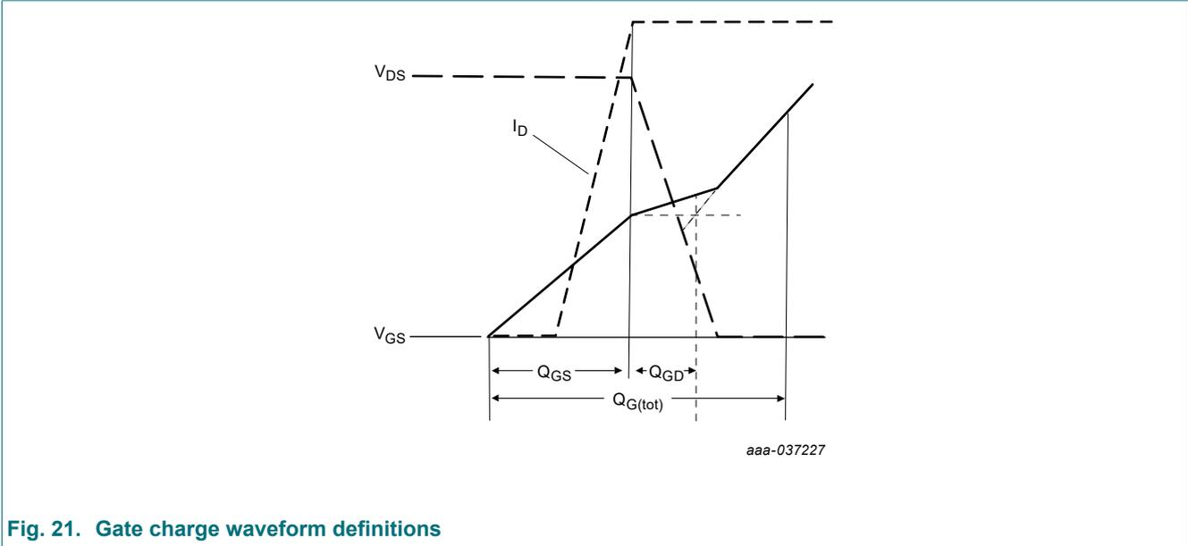
Fig. 21. Gate charge waveform definitions
