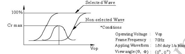
$$Contrast \ ratio(Cr) = \frac{Brightness \ of \ selected \ dots}{Brightness \ of \ non-selected \ dots}$$
