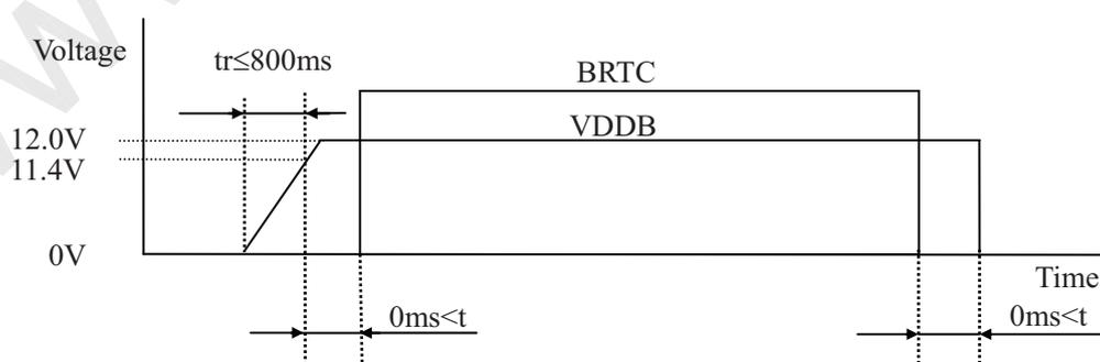
Note1: The backlight should be turned on within the valid period of LVDS signals, in order to avoid unstable data display.
