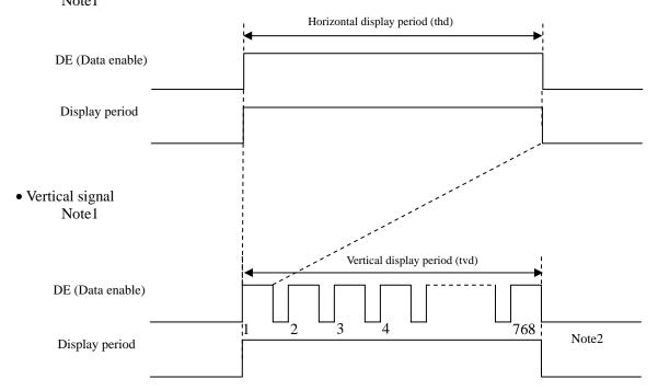
Note1: This diagram indicates virtual signal for set up to timing. Note2: See "**4.9.3 Input signal timing chart**" for the pulse number.
