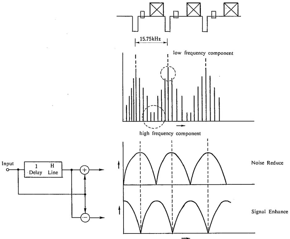
Fig. 6 Video Signal Waveform & Frequency Component
