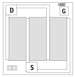
Die Size = 0.052" X 0.052" All Bond Pads  $\geq 0.004$ " Sq. Substrate is also Gate.
