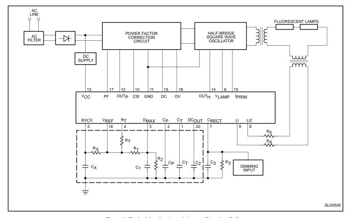
Figure 3. Typical Application: 2-Lamps Dimming Ballast
