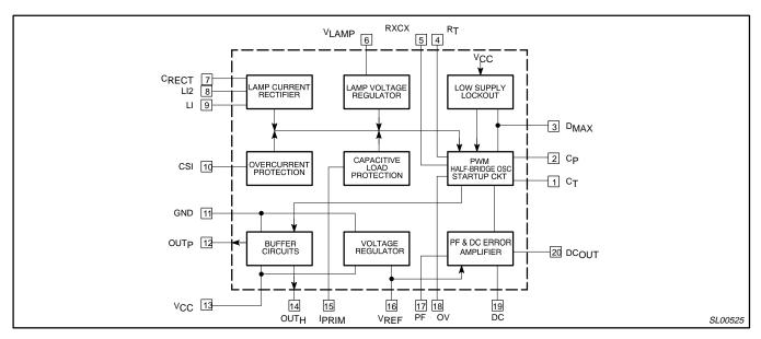
Figure 2. Block Diagram
