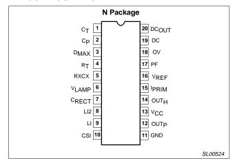
Figure 1. Pin Configuration
