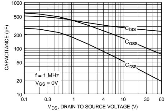
Figure 8. Capacitance Characteristics.
