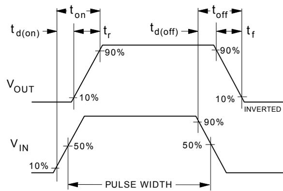
**Figure 12. Switching Waveforms.**
