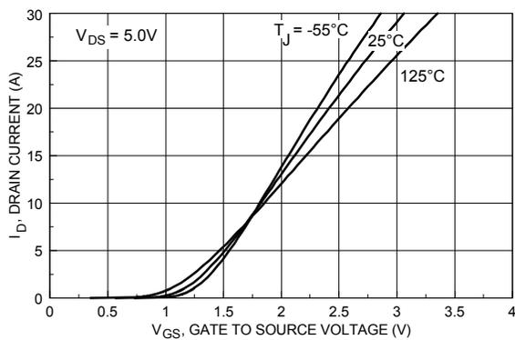
Figure 5. Transfer Characteristics.
