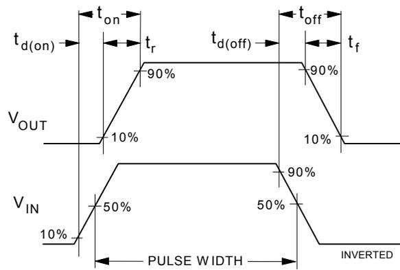
**Figure 12. Switching Waveforms.**
