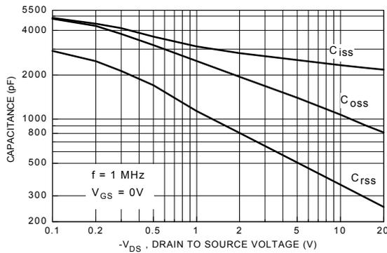
**Figure 9. Capacitance Characteristics.**
