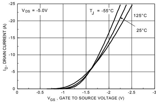
Figure 5. Transfer Characteristics.
