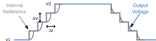
Figure 44. DVS in Forced PPWM Mode Diagram
