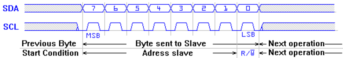
Figure 6. Basic I2C Timings
