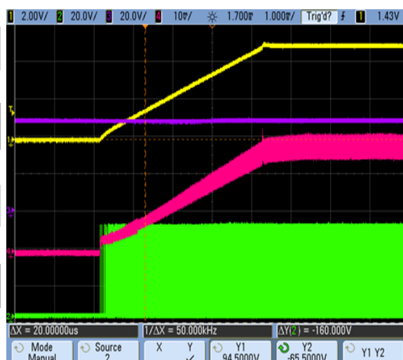
Figure 26. Start-Up Transition at 6A Load (EN = High)
