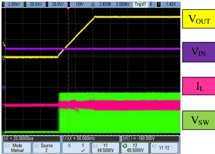
Figure 25. Start-Up Transition at No Load (EN = High)
