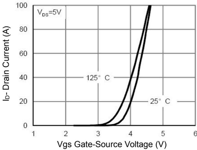
**Figure 2 Transfer Characteristics**
