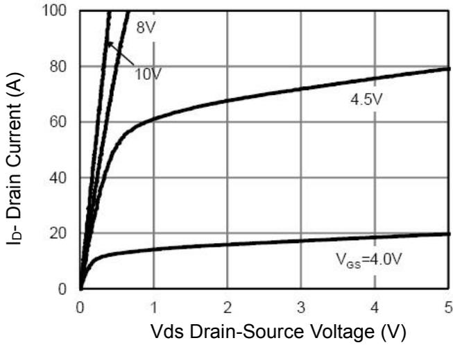
**Figure 1 Output Characteristics**
