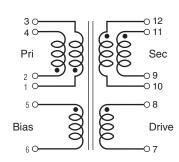
Primary windings and secondary windings to be connected in parallel on PC board
