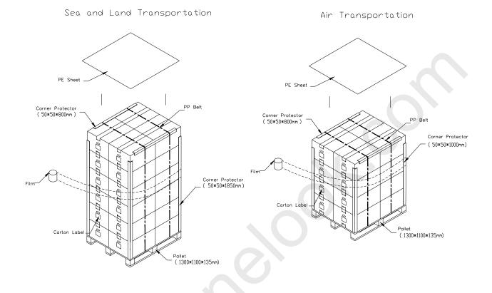
Figure. 9-2 Packing method
