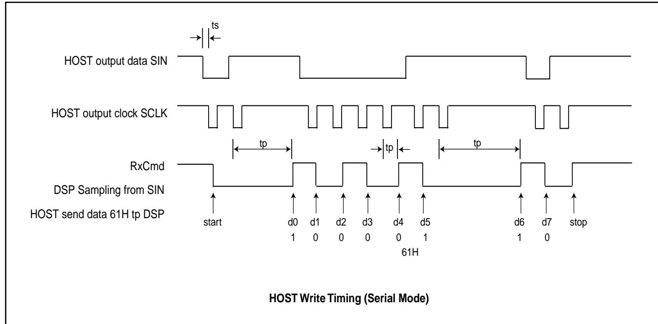
RxCmd become low when start bit is received from HOST and toggle state when MX93521 received each following data bit or stop bit from HOST. Thus, instead of waiting for a fixed period of time (50us) to send a command bit, HOST could send the following command bit as soon as RxCmd toggled from previous state. The delay between the falling edge of SCLK and the RxCmd togglling time is range from 1 us to 50 us
