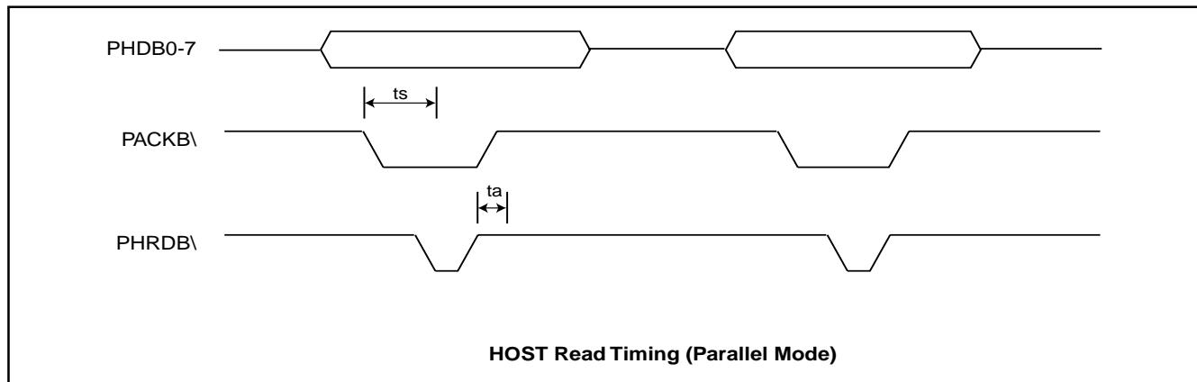
When MX93521 write data to PHDB0-7, PACKB\ will become low. HOST needs to poll the status of PACKB\ continuously. When HOST detect low state on PACKB\, HOST should read out data from PHDB0-7. After HOST read the data from PHDB0-7, PACKB\ will be reset to high.
