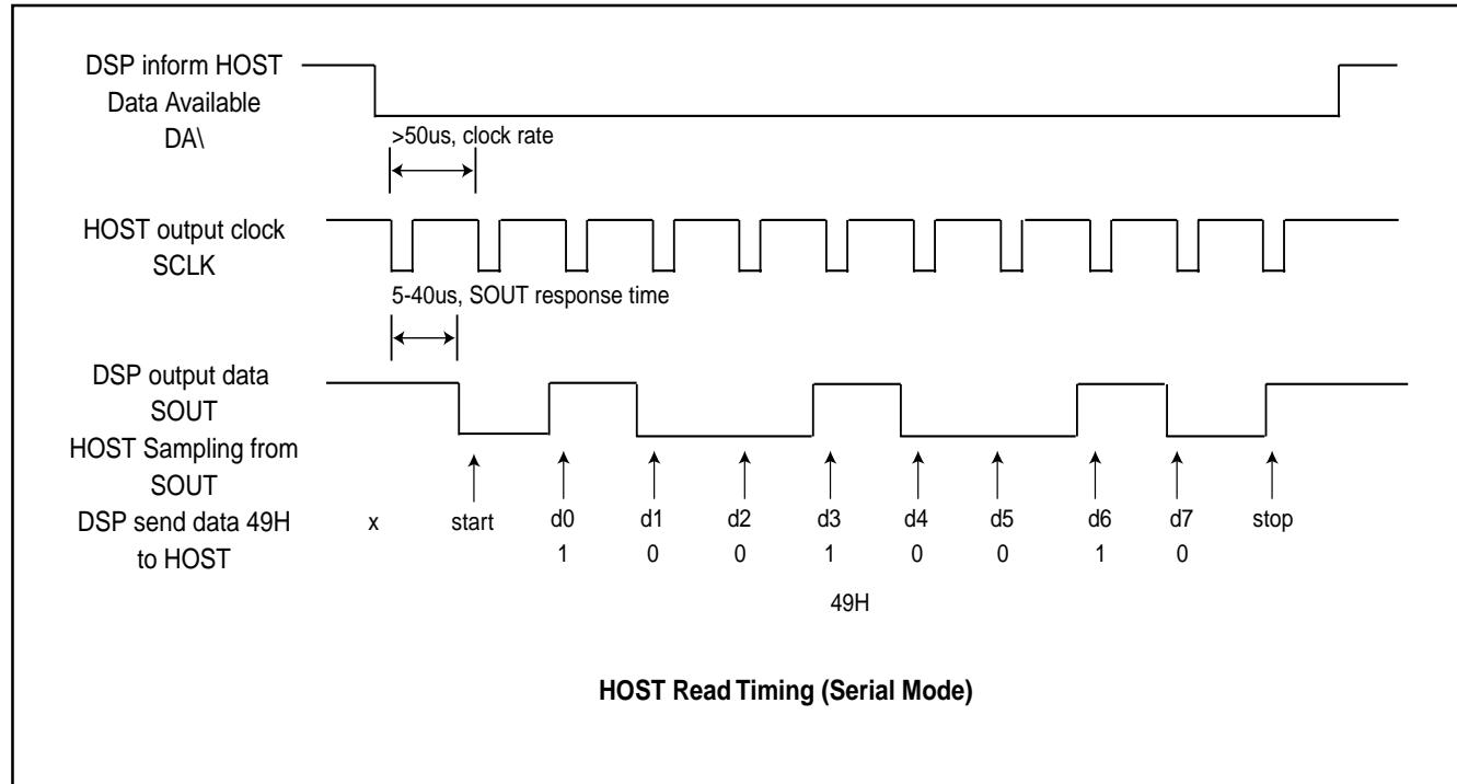
SOUT response time is 5-40us from the falling edge of SCLK
