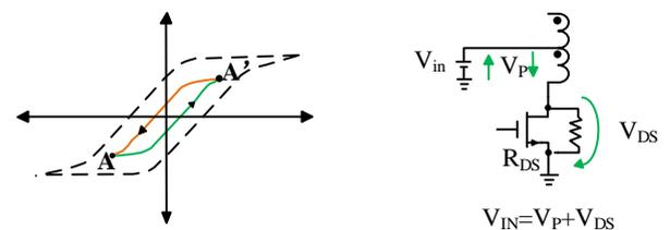
This volt-seconds product is important as it determines the core magnetization during each switching cycle. If the V-t products of both phases are not identical, an imbalance in flux density swing an offset from the origin of the B-H curve. If balance is not restored, the offset increases with each
