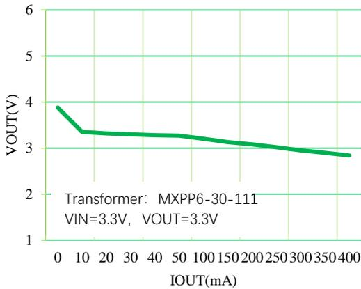
Output voltage vs. load current (3.3V-3.3V)
