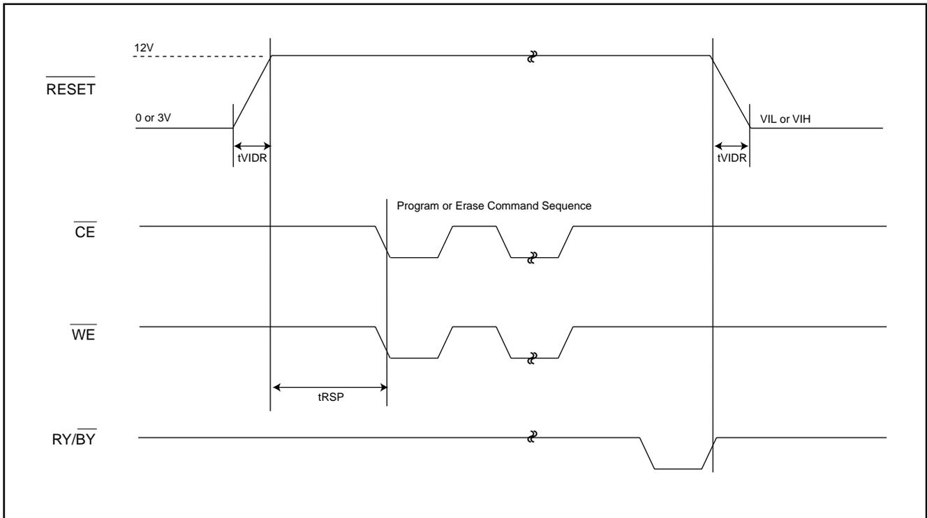
**Fig 20. TEMPORARY SECTOR GROUP UNPROTECTED FLOWCHART**
