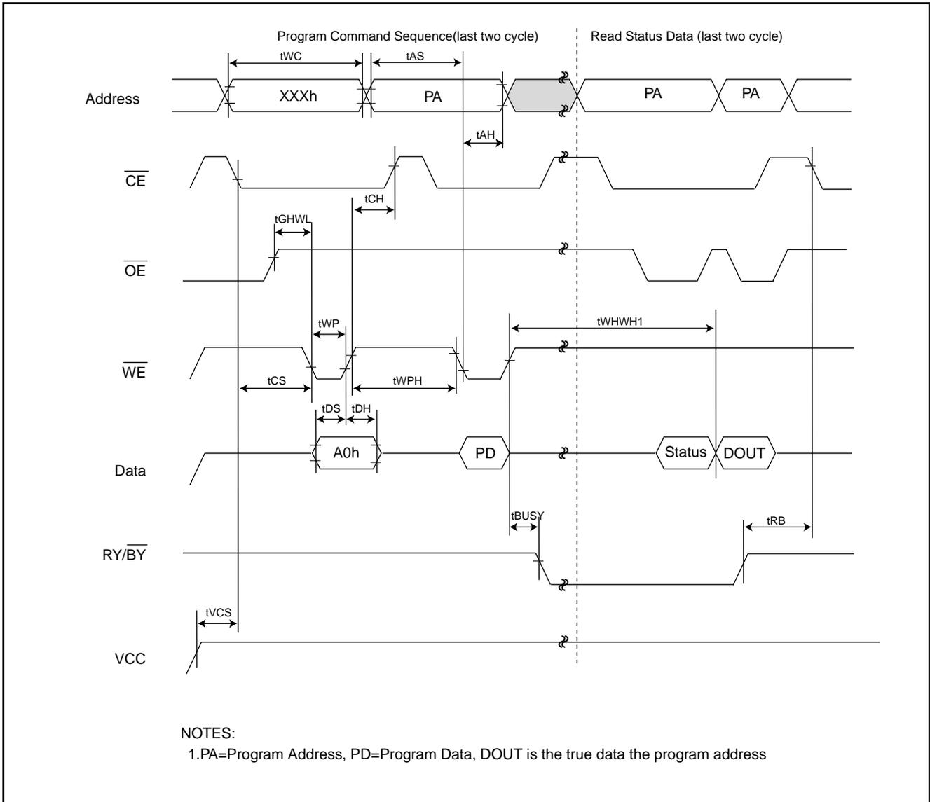
**Fig 10. Accelerated Program Timing Diagram**
