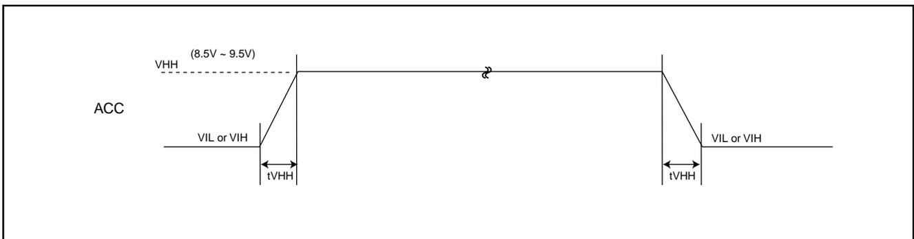
**Fig 11.  $\overline{\text{CE}}$  CONTROLLED PROGRAM TIMING WAVEFORM**
