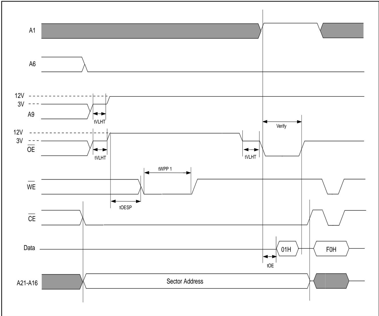
**Fig 15. SECTOR GROUP PROTECTION ALGORITHM (A9,  $\overline{OE}$  Control)**
