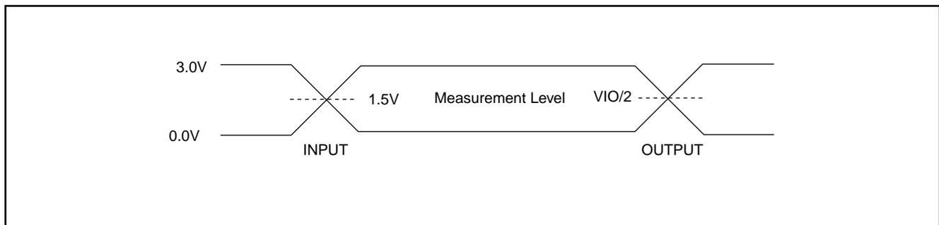
**AC CHARACTERISTICS TA=0°C to 70°C, VCC=2.7V~3.6V**
