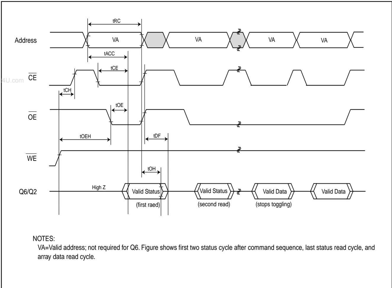
**Fig 15. Toggle Bit Algorithm**
