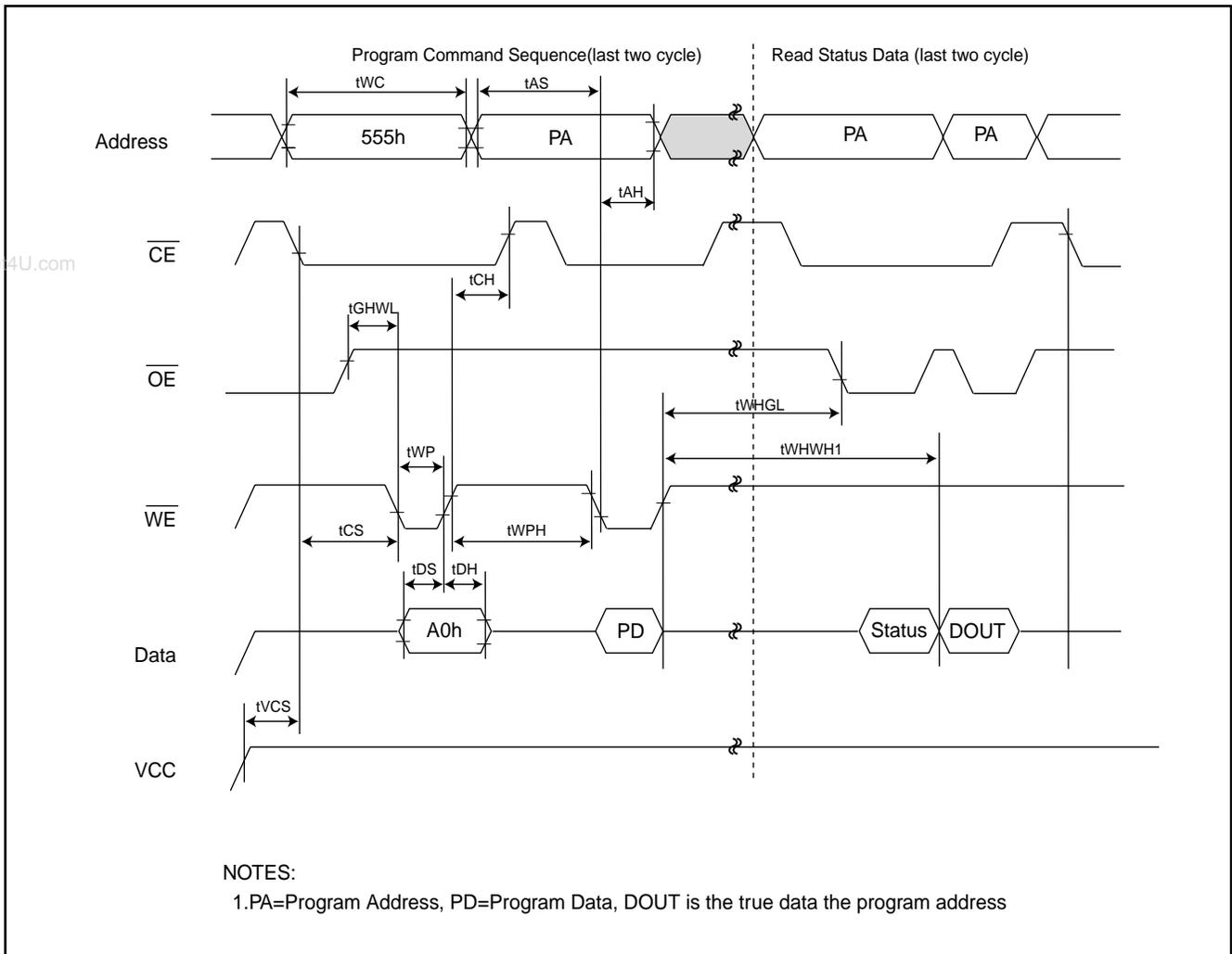
**Fig 7. Accelerated Program Timing Diagram**
