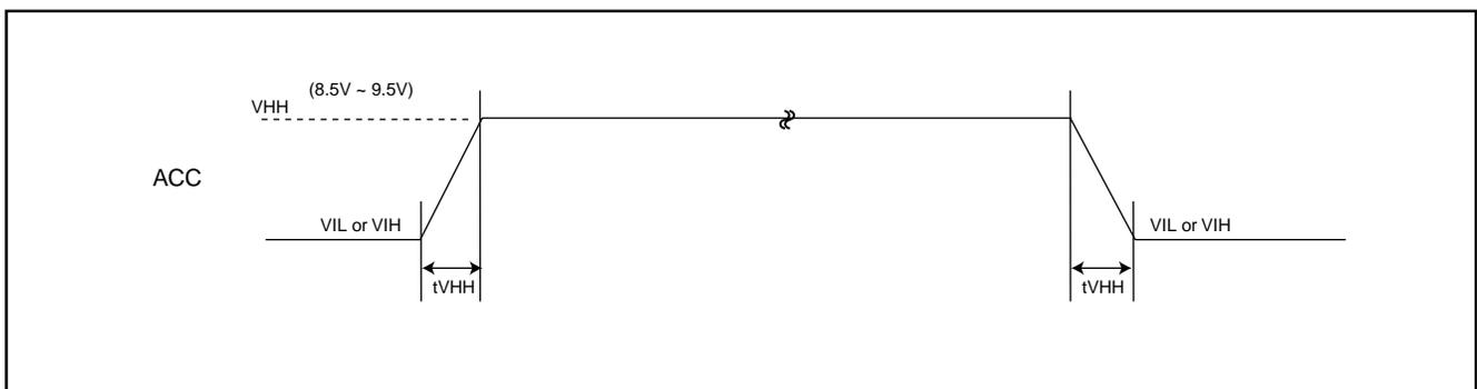
**Fig 8.  $\overline{CE}$  CONTROLLED PROGRAM TIMING WAVEFORM**
