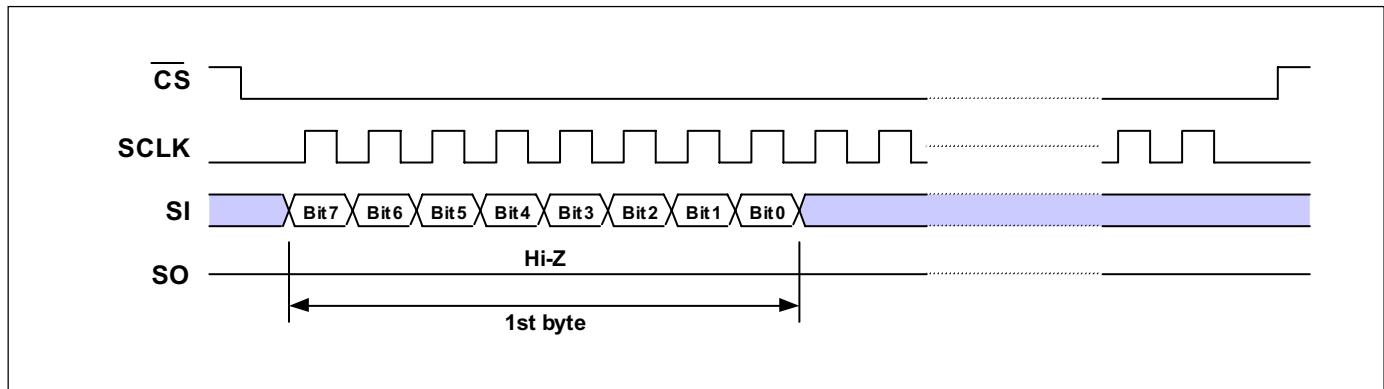
When incorrect command is inputted to this LSI, this LSI becomes standby mode and keeps the standby mode until next CS falling edge. In standby mode, SO pin of this LSI should be High-Z. While  $\overline{CS} = V_{IH}$ , current=standby current, while  $\overline{CS} = V_{IL}$  and commands are issuing, or commands are invalid, current=5mA(typ.) to 15mA(max.).
