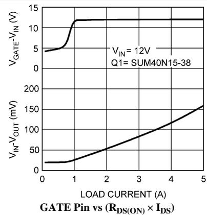
**GATE Pin vs (R<sub>DS(ON)</sub> × I<sub>DS</sub>)**
