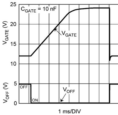
**C<sub>GATE</sub> Charge and Discharge vs OFF Pin**
