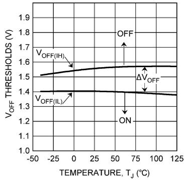
**OFF Pin Thresholds vs Temperature**
