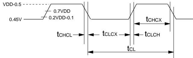
**Figure 32. Clock Signal Waveform for IDD Tests in Active and Idle Modes**
