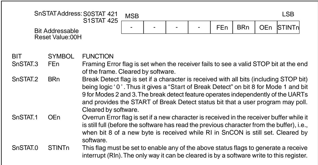
Figure 15. Serial Port Extended Status (SnSTAT) Register
