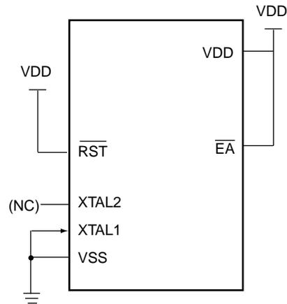
**Figure 33. IDD Test Condition, Power Down Mode**
