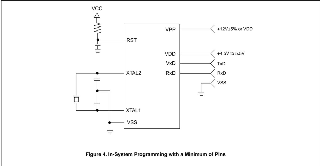
Figure 4. In-System Programming with a Minimum of Pins
