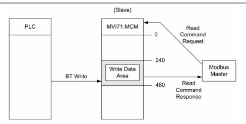
**Ex. 2** -- The next figure shows another example of how to use the Write Data Area; an MVI71-MCM port configured as a Master sends a Modbus Write Command to a slave device. The Modbus Write Command source address in the MVI71-MCM database must be located inside the Write Data Area (between addresses 240 and 479).
