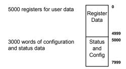
Data contained in this database is paged through the input and output images by coordination of the PLC ladder logic and the MVI71-MCM module's program. Up to 60 words of data can be transferred from the module to the processor at once. Up to 60 words of data can be transferred from the processor to the module. Each image has a defined structure depending on the data content and the function of the data transfer as defined below.
