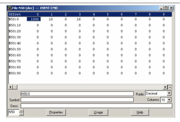
In this example, the module writes (Function 16)10 words from internal address 1000 to address 0 in slave 1 (since we are using blocks 1001 and 2001).
