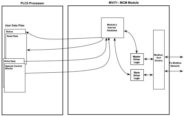
When the side connect interface is used, data is transferred directly between the processor and the module. The module's program interfaces directly to the set of user data files established in the PLC to pass all data between the two devices. No ladder logic is required for data transfer, only the establishment of the data files.
