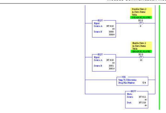
This rung will only execute when a BTR or BTW message is not enabled. This logic is required to alternate between the BTR and BTW messages. When it is time to perform a BTR operation, the 64-word data block will be transferred to N7:410. The remaining branches of the rung then process this data.
