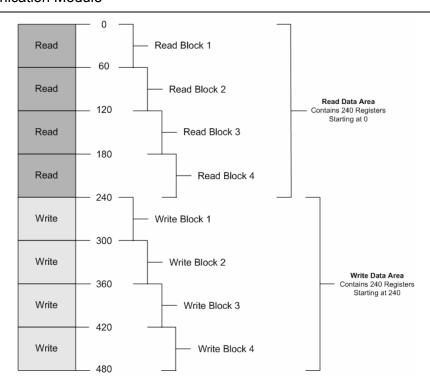
The configuration first creates four possible blocks for each Read and Write area since every block contains 60 registers. Therefore, the Read and Write Block ID generated would be:
