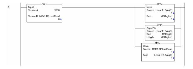
This rung is used to handle Function Code 6 and 16 requests when the module is being used in formatted Pass-Thru mode.
