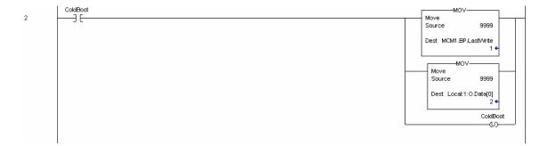
The next four rungs are used to request the slave node status data associated with each master port. Two requests are required for each port in order to obtain the data for the potential 256-slave addresses on a port. The following ladder logic displays what is required to obtain the data for the Modbus Port 1.
