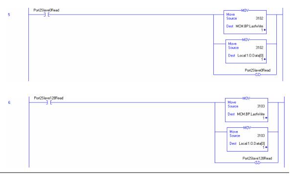
The next rung displays an example of command control. This block of data is passed from the processor to the module to execute a command in a master port's command list.
