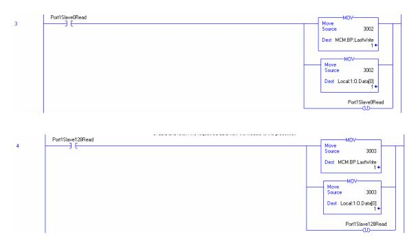
The next two rungs display the logic for the Modbus Port 2 slave status/control data.
