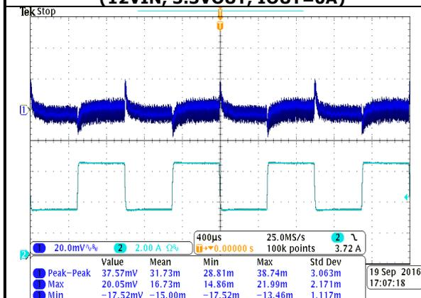
**FIG.31 TRANSIENT RESPONSE (12VIN, 3.3VOUT, 50% to 100% LOAD STEP)**
