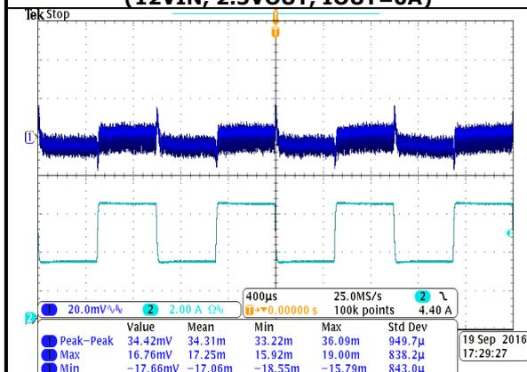
**FIG.25 TRANSIENT RESPONSE (12VIN, 2.5VOUT, 50% to 100% LOAD STEP)**
