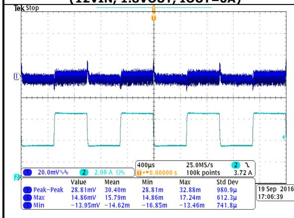
**FIG.19 TRANSIENT RESPONSE (12VIN, 1.8VOUT, 50% to 100% LOAD STEP)**
