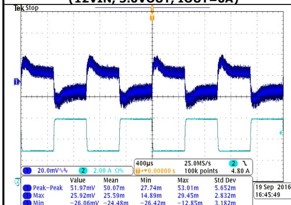
**FIG.37 TRANSIENT RESPONSE (12VIN, 5.0VOUT, 50% to 100% LOAD STEP)**
