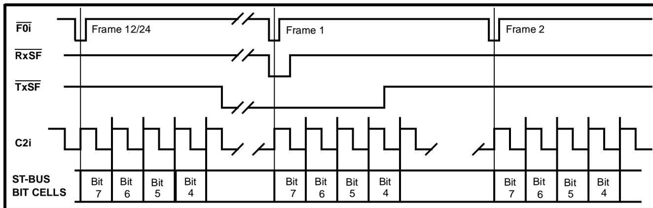
**Figure 12 - Clock & Frame Alignment for ST-BUS Streams**
