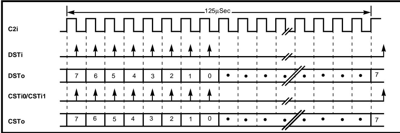
Figure 3 - ST-BUS Timing
