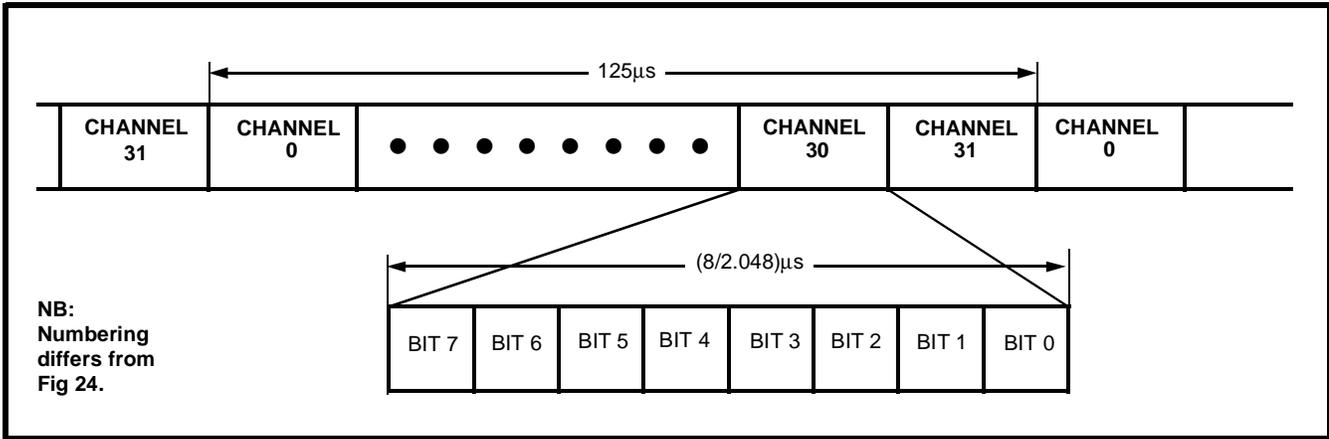
Figure 23 - Format of 2048 kbit/s ST-BUS Streams
