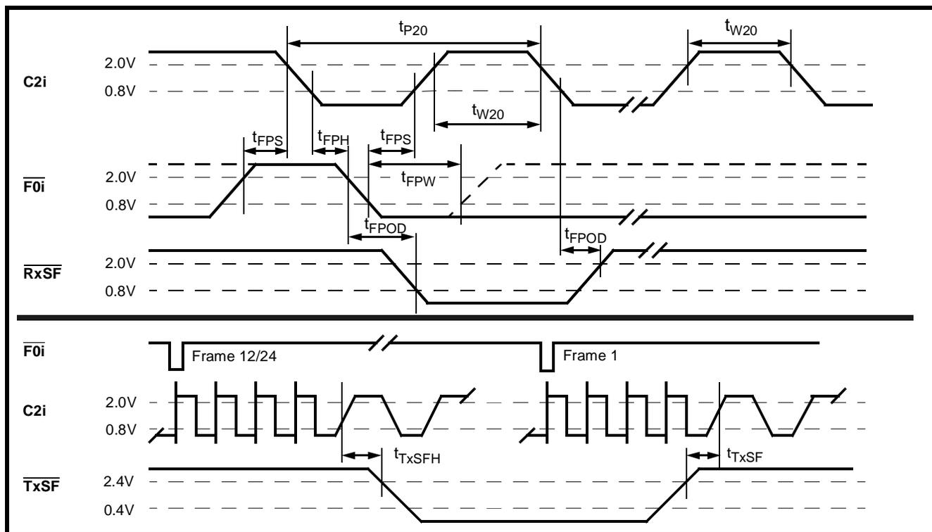
**Figure 13 - Clock & Frame Pulse Timing for ST-BUS Streams**
