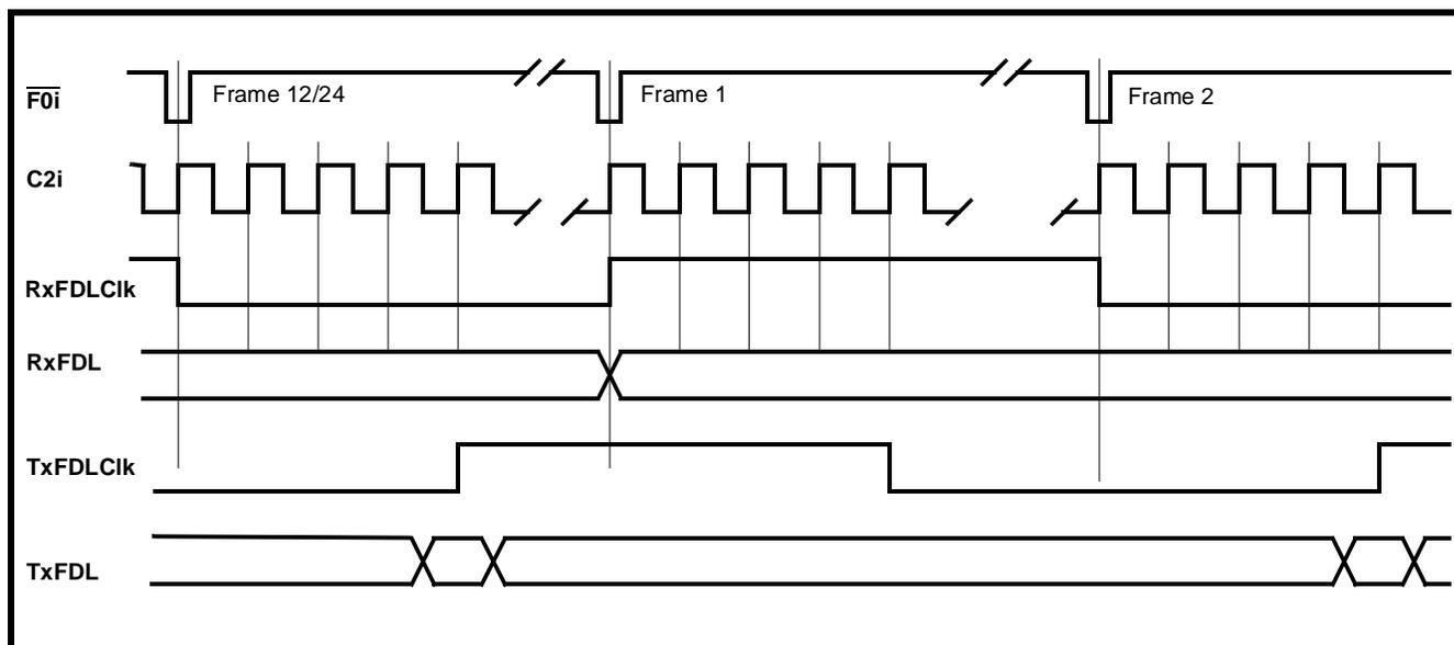
**Figure 21 - Clock & Frame Alignment for RxFDL and TxFDL**
