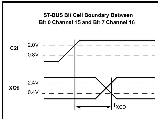
**Figure 16 - XCtl Timing**
