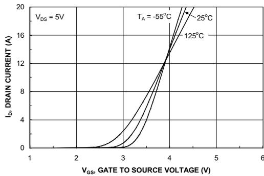
Figure 15. Transfer Characteristics.
