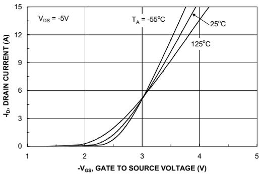
Figure 5. Transfer Characteristics.
