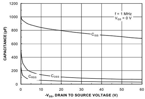
Figure 8. Capacitance Characteristics.
