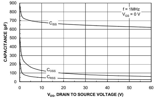
Figure 18. Capacitance Characteristics.
