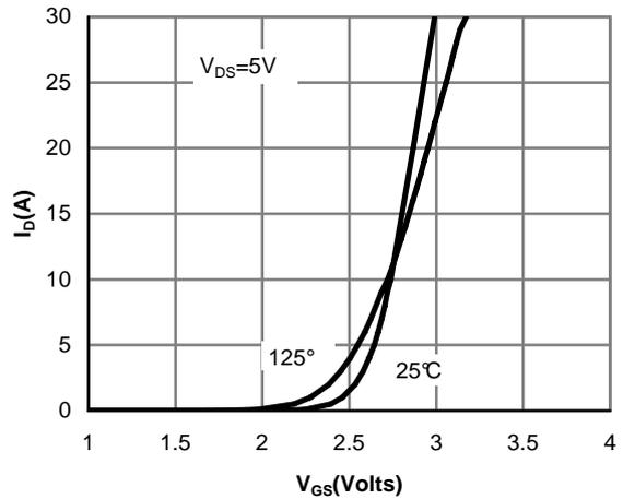
Figure 2: Transfer Characteristics
