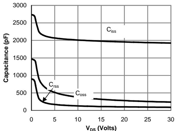
Figure 8: Capacitance Characteristics
