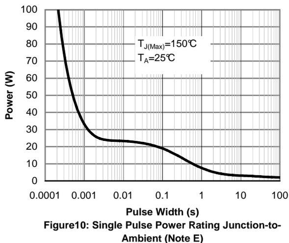
Figure 10: Single Pulse Power Rating Junction-to-Ambient (Note E)
