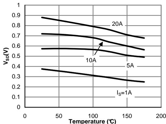
Figure 13: Diode Forward voltage vs. Junction Temperature
