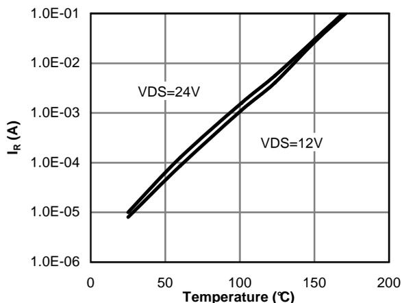
Figure 12: Diode Reverse Leakage Current vs. Junction Temperature
