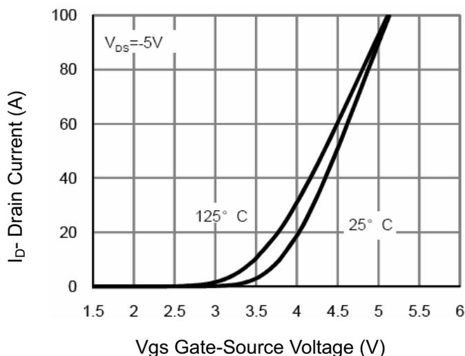
**Figure 5 Transfer Characteristics**
