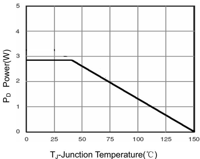
**Figure 1 Power Dissipation**
