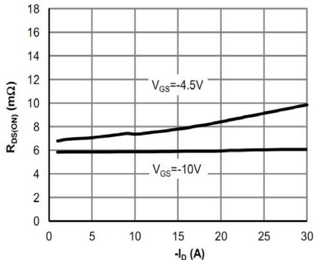
**Figure 4 Drain-Source On-Resistance**
