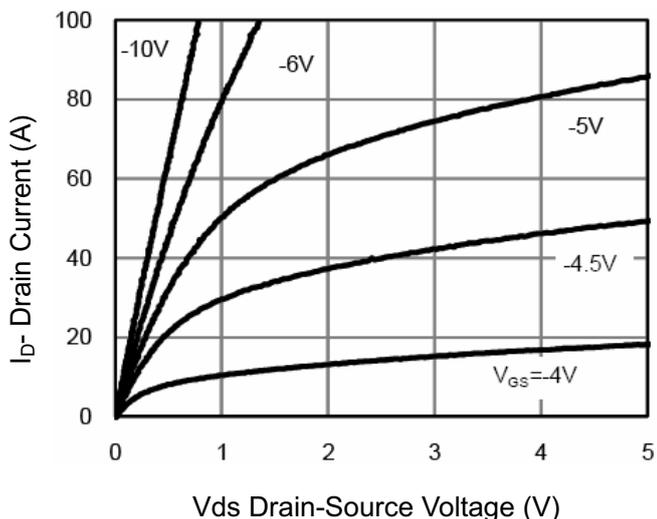
**Figure 3 Output Characteristics**
