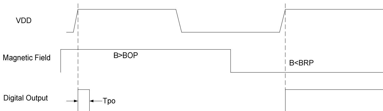
Note: VDD power on raise<1us, time of output start up high level T<sub>po</sub><100us when B>Bop
