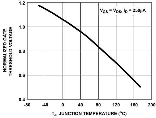
**Figure 11. Normalized Gate Threshold Voltage vs Junction Temperature**
