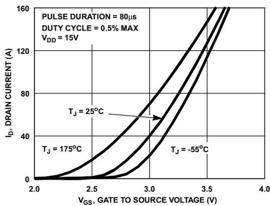
**Figure 7. Transfer Characteristics**
