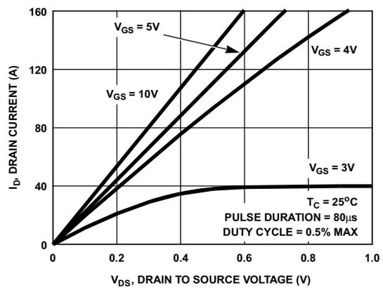
**Figure 8. Saturation Characteristics**
