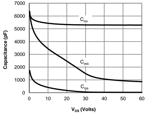
Figure 8: Capacitance Characteristics
