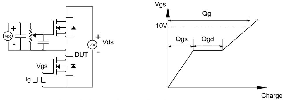
Figure B: Resistive Switching Test Circuit & Waveforms
