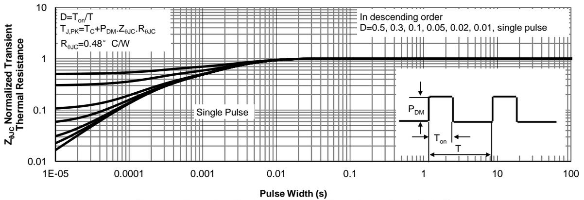
Figure 11: Normalized Maximum Transient Thermal Impedance (Note F)
