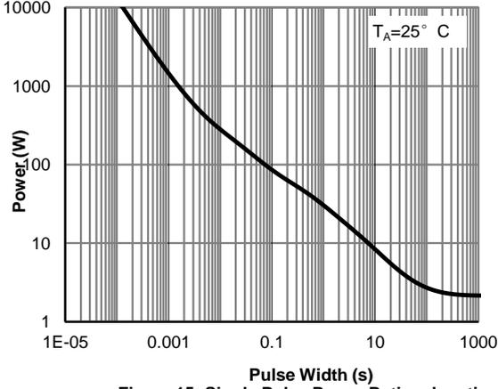
Figure 15: Single Pulse Power Rating Junction-to-Ambient (Note H)
