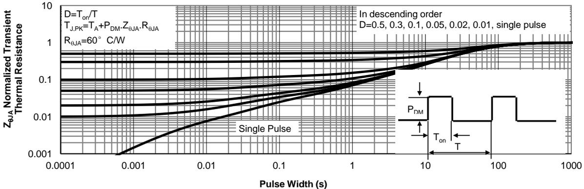
Figure 16: Normalized Maximum Transient Thermal Impedance (Note H)
