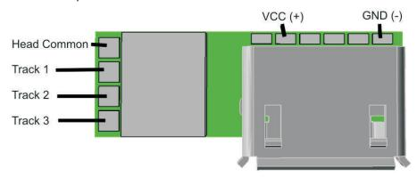
MSRv007 requires at least 2.8 Volts to work correctly and a maximum of 3.8 volts. Please read the MSRv007 datasheet for complete information.
