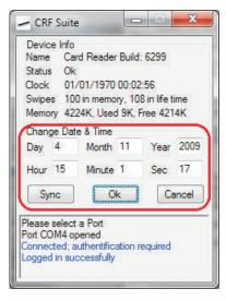
**Clock** - When you power on the MSRv007, it starts from 00:00:00 1/1/1970 GMT. 00:00:00 is set exactly when the light blinks twice. You can change the device date and time by pressing this button. You will be prompted with 6 text boxes in which you can write the date and time required (as in the picture on the left)
