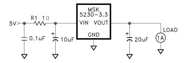
For a given continuous maximum load of 1 amp, R1 can be selected to drop the voltage seen at the regulator to 4V. This allows for the output tolerance and dropout specifications. Input voltage variations (5V) also should be included in the calculations. The resistor should be sized according to the power levels required for the ap-
