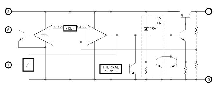
Schematic shown for fixed output voltage versions
