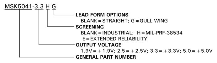
The above example is a +3.3V, MIL-PRF-38534 Class H regulator with gull wing leads.
