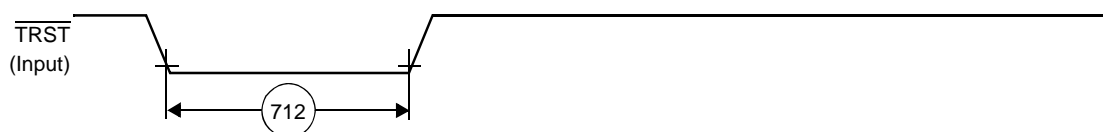
Figure 25. \overline{\text{TRST}} Timing Diagram
