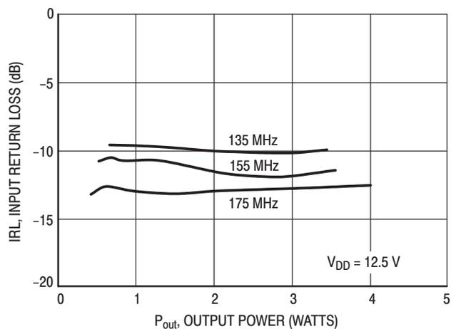
Figure 21. Input Return Loss versus Output Power
