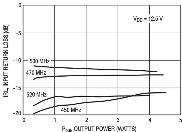
Figure 3. Input Return Loss versus Output Power
