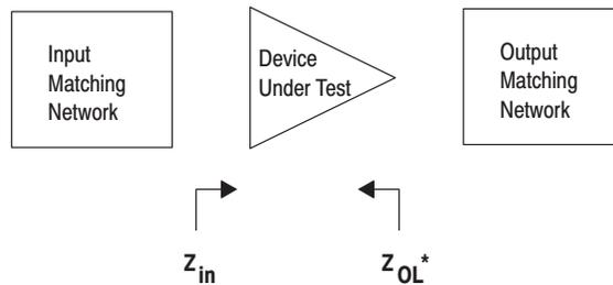
Figure 28. Series Equivalent Input and Output Impedance
