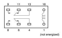
Note The coil has no polarity.
