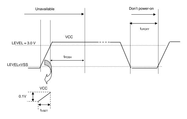
Note: A start-up delay of 1ms is required after power-on.
