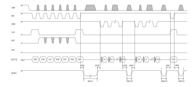
Note: Data Read Cycle would end without a stop command (F0h) after reading the end address. At that time, RD/BY signal would be LOW once for tBSYS.
