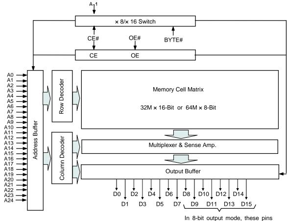
In 8-bit output mode, these pins are placed in a high-Z state and pin D15 functions as the A-1 address pin.
